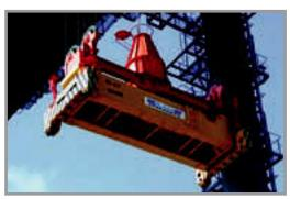
Ram ship-to-shore quay crane spreader
