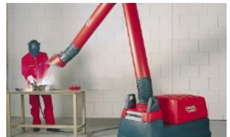
Individual Mobile Extraction Workstation (for controlling hazardous fume and gases during welding)
