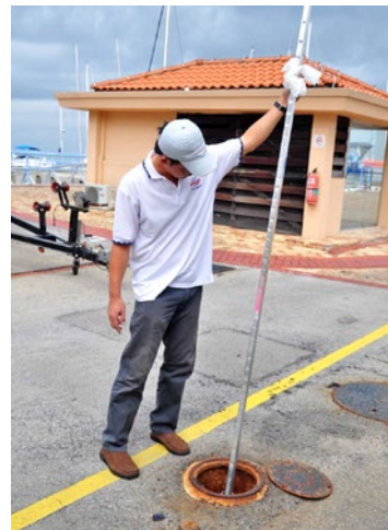
(Left) Present process: Staff using a measuring stick to determine the level of fuel outdoors.
