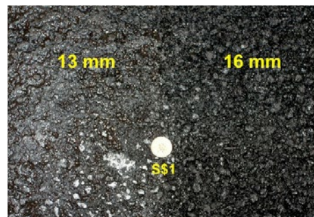
Comparison of New Mixes, against S$1 coin
