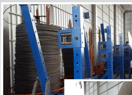
▲ Coils are fed into the automated machine
