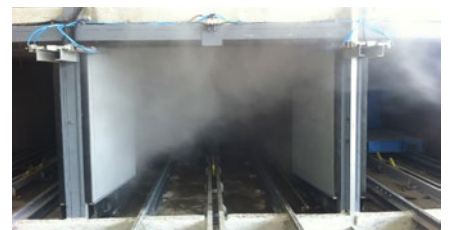
Curing chamber, where the tunnel segments will be transferred and steam will be emitted to accelerate curing of concrete.
