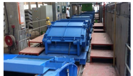
Tunnel Segment Moulds in its respective work-stations
